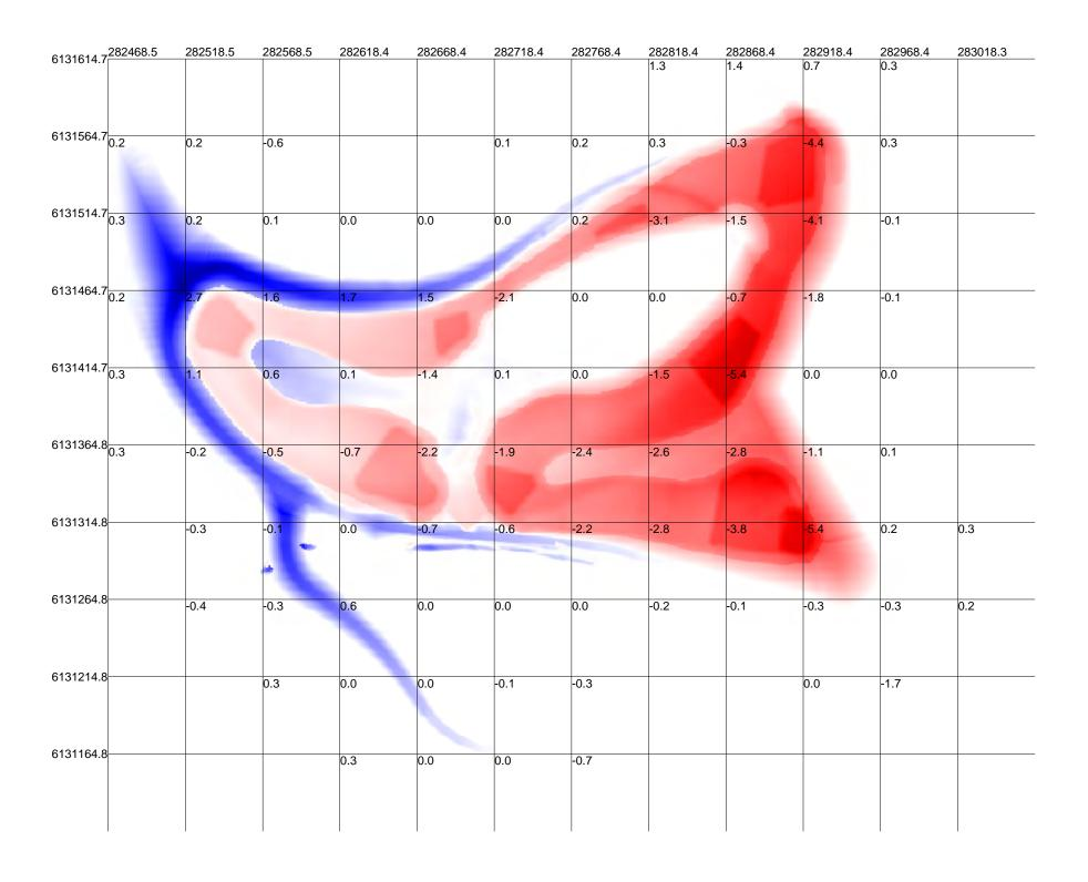
Area: Site Perimeter (Batter Edges), Intersection Point: Lower Left Corner, X Grid: 164, Y Grid: 164, Average Haul Distance: 361.8 m
