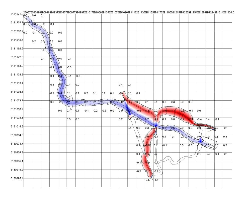
Area: Site Perimeter, Intersection Point: Lower Left Corner, X Grid: 65, Y Grid: 65, Average Haul Distance: 199.1 m
